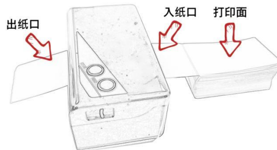
②无支架安装 Installation without support
